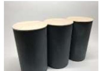
When the glue is dry, trim the excess overhang off using a razor blade and then lightly sand to make sure the end is the same diameter as the pipe and paint.
