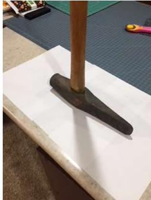
This item is a rail jack, primarily used to lift the track so that a tie could be easily replaced or tamped up to level the rail. The section gang would remove some ballast beside the tie of interest, place a tie plate on the ballast and then set the jack in place with the foot on the front of the jack under the rail. The design of the jack is such that the ram would rise out of the top making it useful for lifting other items as well.
